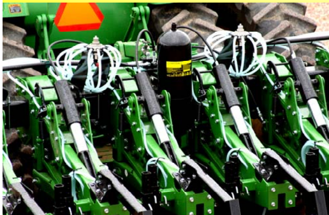
Hydraulic Trip/Reset units keep you moving in even the rockiest conditions
