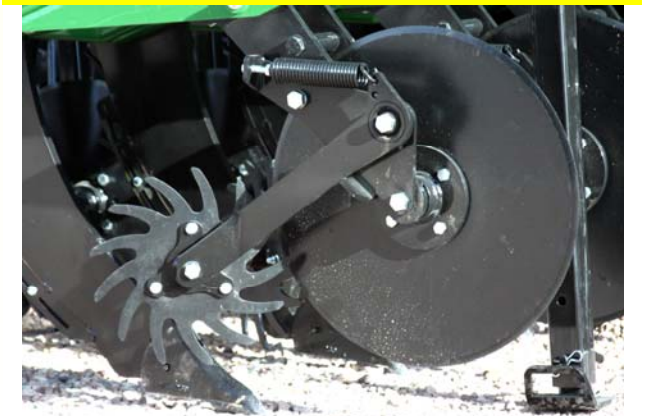
SPRING-LOADED ROW CLEANERS WILL CLEAR THE SEED BED SURFACE
