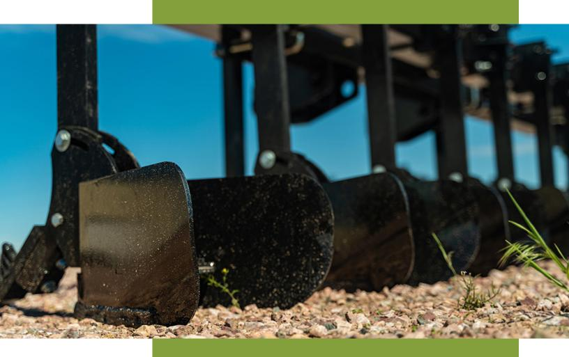
Single clamps are made for 7" or 7"x 5" bars, and the ditcher wings are made of sturdy 1/4" plate with hard surfacing on the leading edges.
